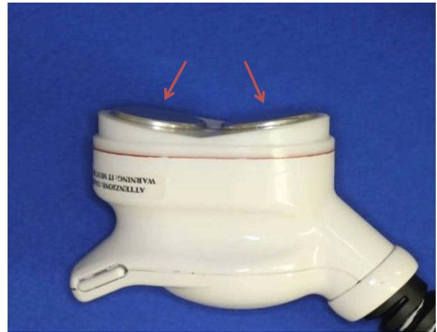
**Figure 1:** MC1 device. The MC1 device has an ultrasound and a zonal massage handpiece. The ultrasound handpiece with angled, nonfocused emitters deliver 1 MHz ultrasound. In modulated emission mode, the nonfocused beams create a slightly focused ultrasound field within the tissue at the point where the beams overlap
